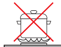
Bottom too small for this burner
